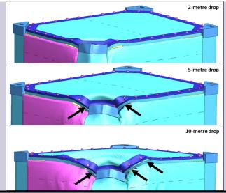
FEA Modelling of a dropped 2m Box, showing progressive damage with height
