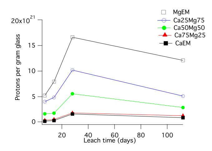
Proton content of altered layer shows clear compositional dependence on Mg content of glass.
