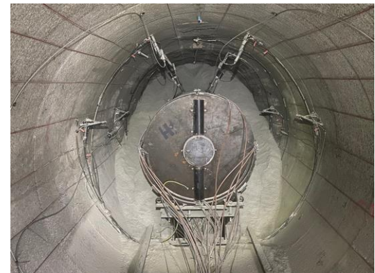
HotBENT experiment, Heater # 1 instrumented and partially backfilled. Reproduced from GTS website
