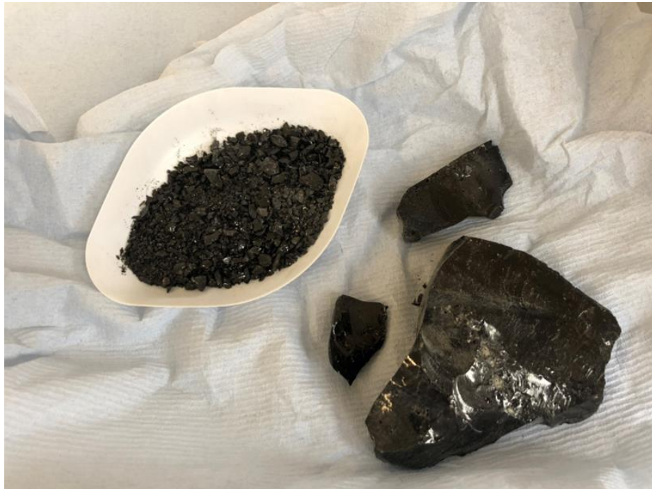
'Mixture Windscale' 25 wt% magnesium non-oxidising (Magnox) waste loaded boro-alumino-silicate glass (MW25) – Nuclear Waste Services
